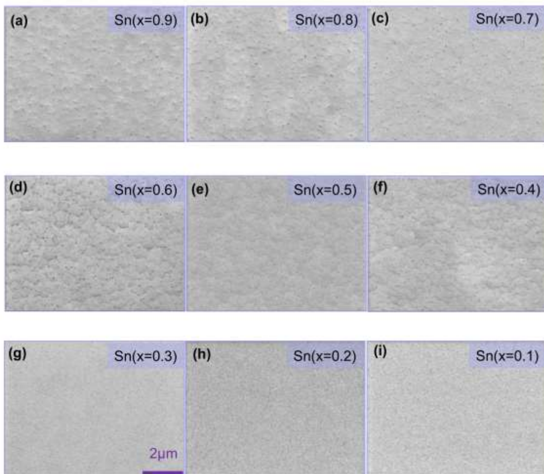
Figure S20 (a-i). Scanning electron microscope (SEM) images with the same magnification (30 kx) of \text{PEA}_2\text{Sn}_x\text{Pb}_{1-x}\text{I}_4 ( x=0.1\dots ) polycrystalline films show that the grain size becomes smaller with the Pb ratio increasing.
