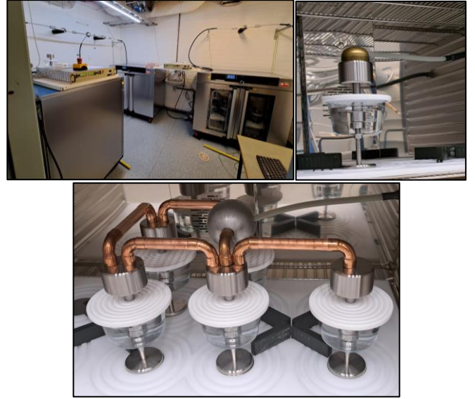
Fig. 2. ALTs test system developed at Tampere University, consisting of the test chambers in the top corner and the test cells at the lower row.
