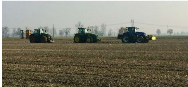
Fig. 1: Tractor under testing followed by the two braking units connected through ropes during a repetition of the transient procedure.
