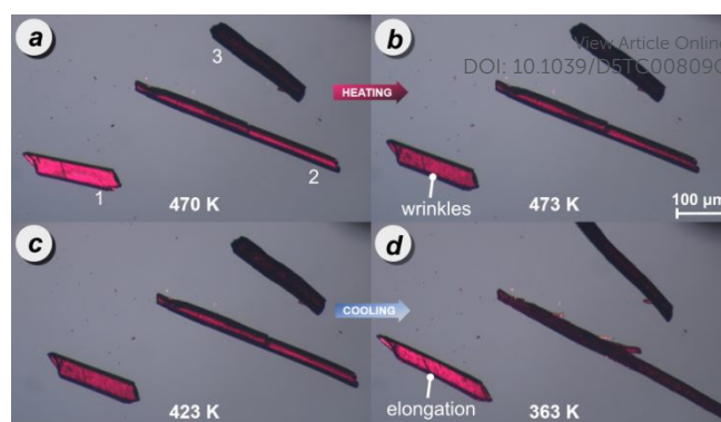
Figure 2. Hot stage microscopy of PDI-C 6 crystals during the heating cycle: (a) phase I at 470 K, (b) transition from phase I to phase II at 473 K; and during cooling cycle: (c) phase II at 423 K, (d) transition from phase II to phase I at 363 K, reshaping the crystals. Additional images are provided in Figures S18 and S19 of the SI.
