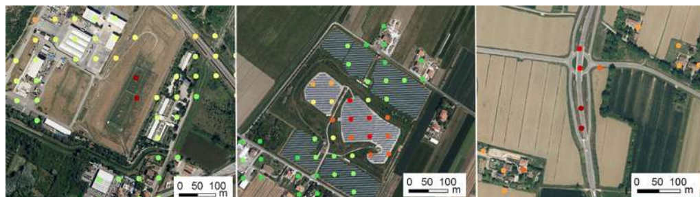
Figure 11. Examples of areas exhibiting anomalous vertical ground velocities resulting from anthropogenic activities or infrastructure are identified as outliers. On the (left), a landfill; in the (center), a photovoltaic solar park; and on the (right), a viaduct.
