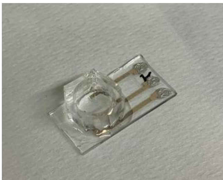
Fig. S7. OECT equipped with a PDMS well to analyze 250 \mu\text{L} of sample.
