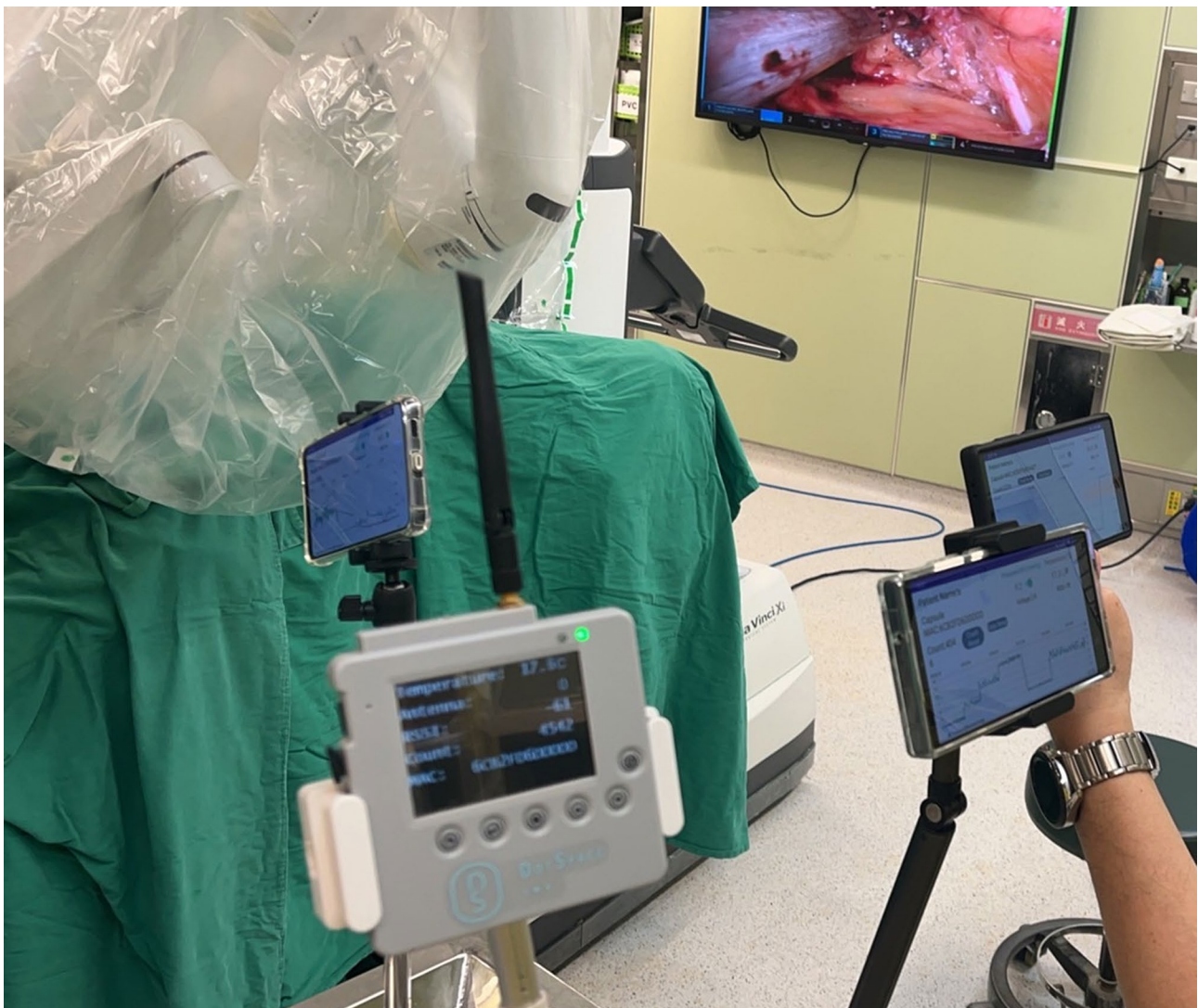
Fig. 2 Multiple Bluetooth receivers were used to collect pressure data at different positions to complete all the transmission tests and the continuous IAP monitoring tests
