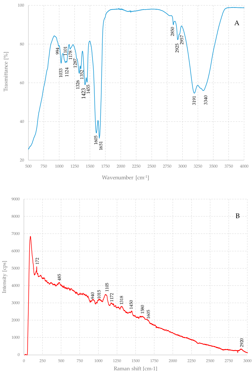
Figure 3. IR (A) and Raman (B) spectra of the dehydrated pristine hybrid hydrogel.
