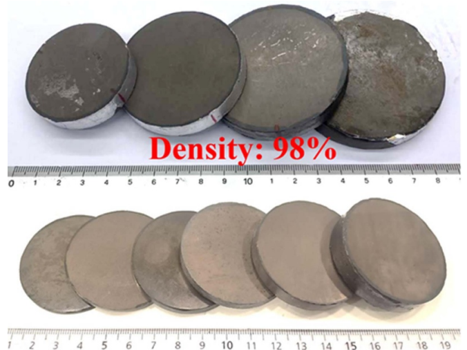
Figure 2. Photograph of the \text{MgB}_2 discs prepared by the spark plasma sintering.
