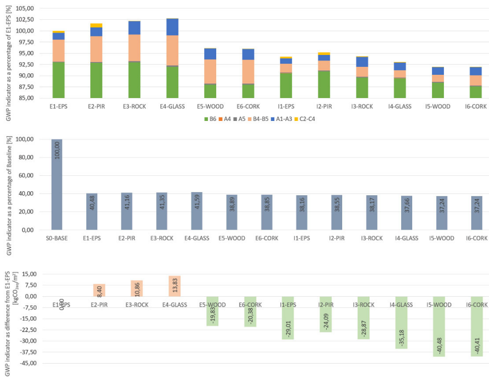
Figure 4: Results expressed at building-scale: at the top, carbon footprint assessment as a percentage of the E1-EPS scenario; in the middle, comparison with the baseline (no interventions); at the bottom, comparison expressed in terms of kgCO 2eq /m 2 .
