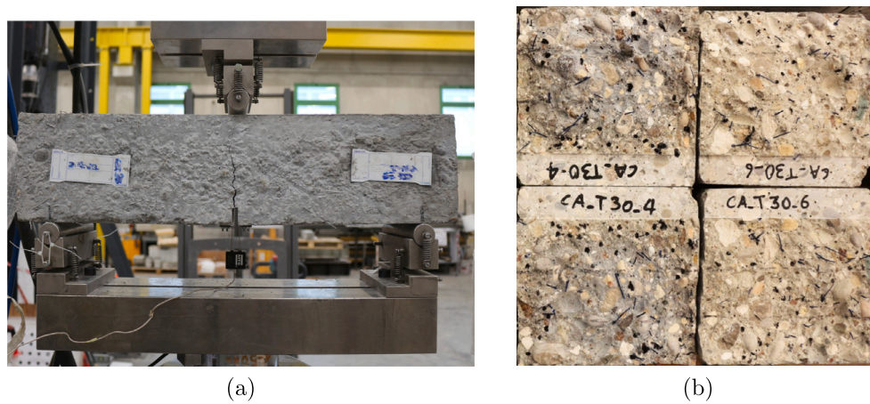
Fig. 2. (a) Crack observed at the end of one of the bending tests and (b) distribution of the fibers in the cross sections separated by the crack in the specimens T4 (left) and T6 (right). Fibers are marked with black dots.
