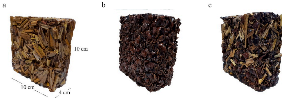
Fig. 2. Composite samples 10 cm × 10 cm × 4 cm made of bio-aggregates and sodium silicate solution: a) A. donax -based; b) hazelnut shells-based; c) mixture-based.
