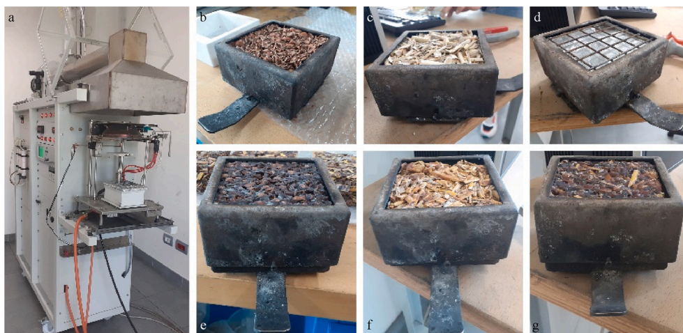
Fig. 4. Test to evaluate the fire reaction by exposing the materials to a constant heat source. a) Cone calorimeter; samples into the metal mould ( 10\text{ cm} \times 10\text{ cm} \times 4\text{ cm} ) before the test: b) hazelnut shells H, c) A. donax A; d) air-dried sodium silicate solution S; e) hazelnut shells-based composite HS; f) A. donax -based composite AS; g) mixture-based composites AHS.
