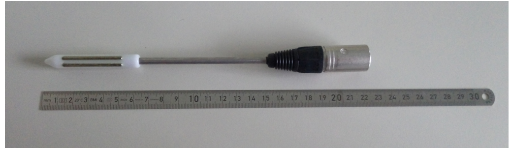
Figure 1. Electroejaculator probe. Total length 22 cm, portion with two electrodes length 6 cm and with a diameter of 1.27 cm.
