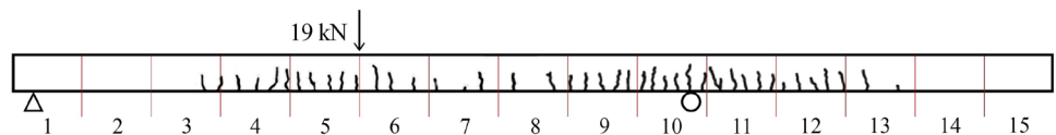
Fig. 22 Second damage scenario for the concrete beam corresponding to an applied load equal to 19 kN (step 9 in [34])
