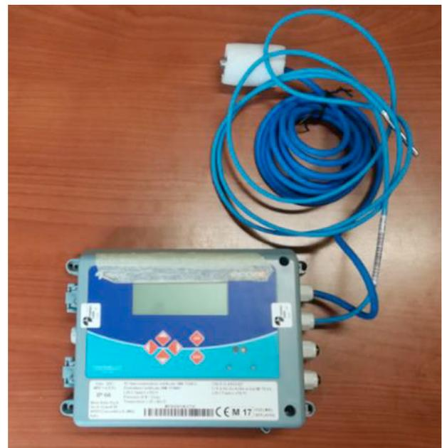
Figure 2. External view of the NG volume converters under test.
