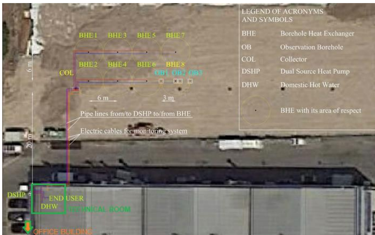
Figure 7. Map of the BHE field in the Tribano demo-site. Temperature sensors are located in OB 1,
