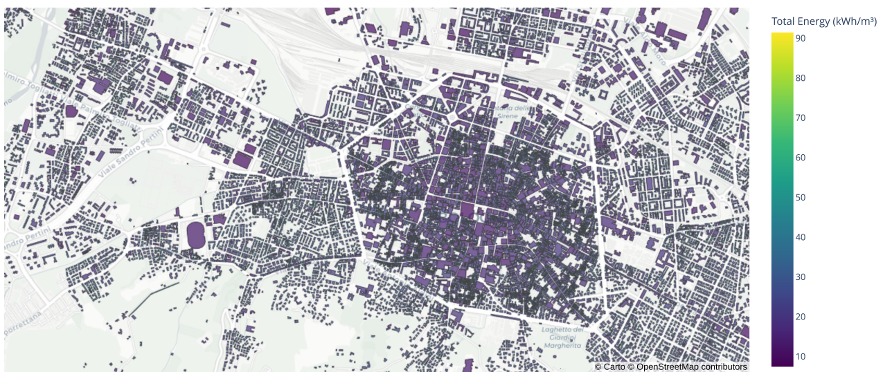
Figure 4. Simulated annual energy consumption ( \text{kWh}/\text{m}^2 ) for a portion of the building stock. Buildings are colored according to their annual energy use per square meter. Administrative zone and street names are shown in Italian for geographic reference.
