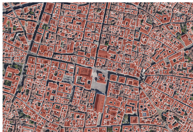
Figure 1. Snippet image of building footprint polygons in shapefile format, derived from the Building Parcels dataset, illustrating the spatial representation of some buildings used as input data in this work.
