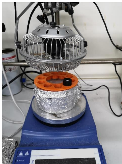
Figure S3: Left panel: Blue LEDs photoreactor used for reactions. Right panel: Emission spectrum of the 465 nm LED strip used in this reactor.
