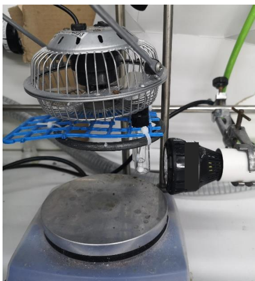
Figure S5: 456nm EvoluChem™ setup.
