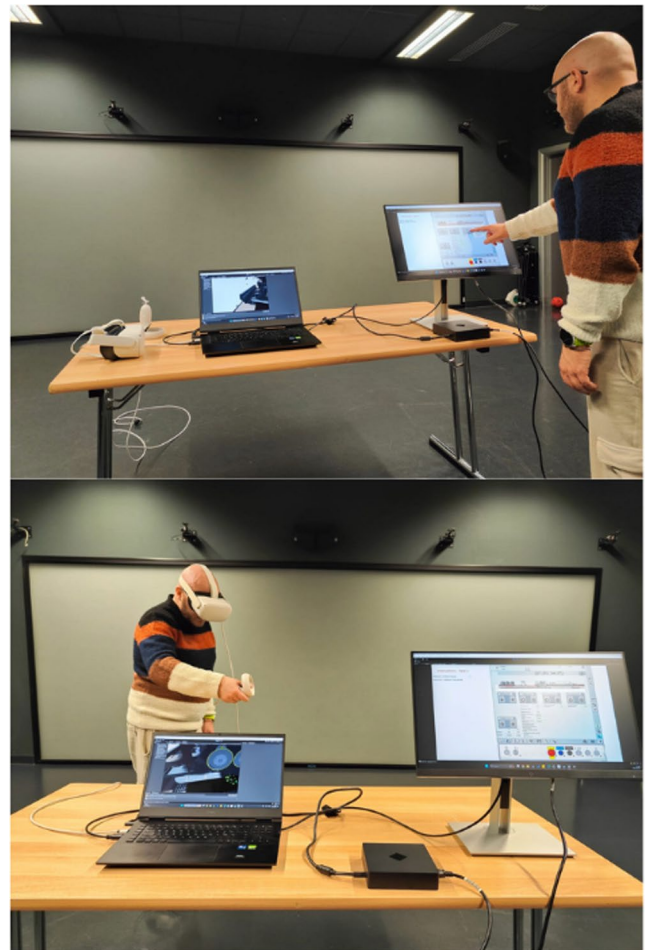
Fig. 7 Execution of the test by a user: the top section shows an example of interaction with the HMI, while the bottom section displays the user interacting in VR
