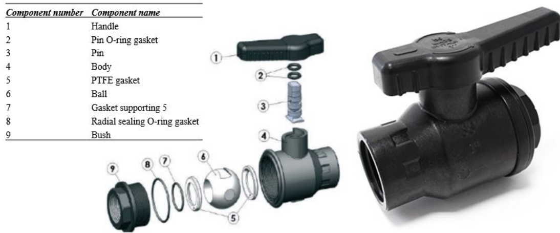
Figure 6. Example of a valve variant and its components
