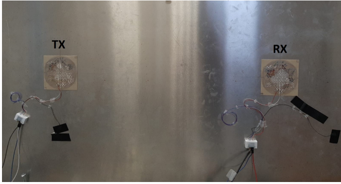
Fig. 5. Experimental setup: Discrete-FSAT bonded on the 1 mm thick aluminium plate, at a distance of 50 cm along the 0° direction
