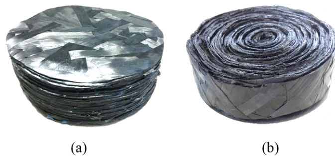
Figure 3: a) ASMC stacked with fiber orientation parallel to the platform interface; b) ASMC stacked with fiber orientation orthogonal to the platform interface.
