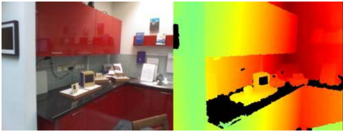
Fig. 21: The 71st frame of the Red Kitchen testing sequence from 7-Scenes [25]. Here, our relocaliser initially produces a pose that is within 5\text{cm}/5^\circ of the ground truth, but ICP against the fused 3D model then refines it to a pose that is further from the ground truth. The ultimate cause of this is slightly inaccurate ground truth poses in the training sequence, leading to InfiniTAM fusing an imperfect 3D model, which then affects the pose to which ICP converges.
