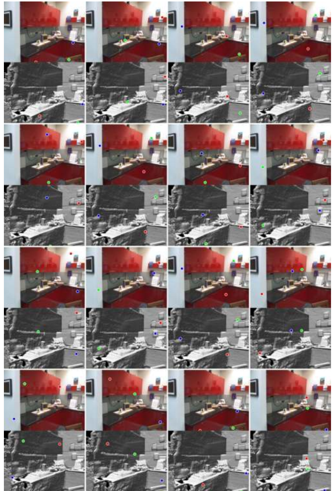
Fig. 23: The top 16 pose candidates (left-to-right, top-to-bottom) corresponding to the failure case from the Red Kitchen scene shown in Figure 21. The coloured points indicate the 2D-to-3D correspondences that are used to generate the initial pose hypotheses. Note that in this case, the relocalised pose before ICP was within 5\text{cm}/5^\circ of the ground truth, but that the 3D model seems somewhat eroded in comparison to the original input images. This is caused by slightly inaccurate ground truth poses in the training sequence, leading to InfiniTAM fusing an imperfect 3D model, which then affects the pose to which ICP converges.
