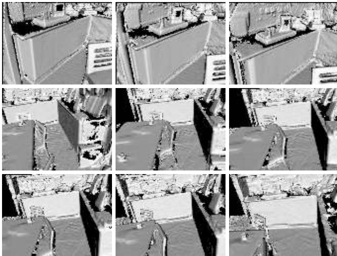
Fig. 22: The process of fusing the Red Kitchen training sequence from 7-Scenes [25] using InfiniTAM (left-to-right, top-to-bottom). Initially (top-left), the brown box on the worktop is correctly reconstructed, but as the fusion process proceeds, it gradually becomes more and more eroded. This is ultimately caused by slightly inaccurate ground truth poses in the dataset, causing points that should be fused into the same place in the model to be fused at a slight offset from each other, with the results as shown (bottom-right).
