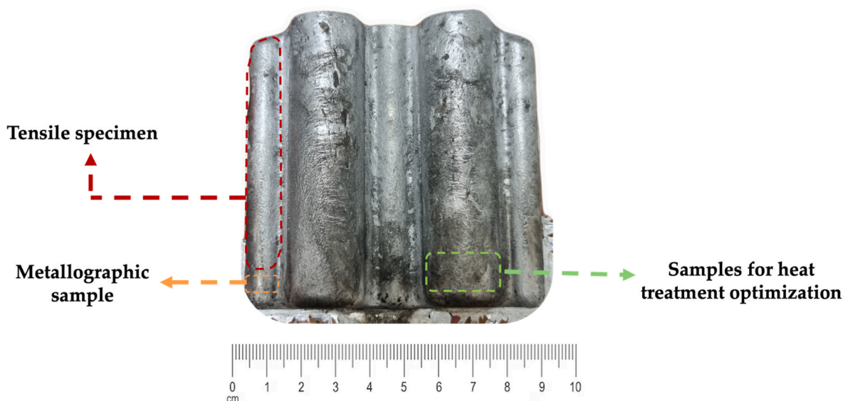
Fig. 1. Extraction zones from a EN 45500 casting of samples used for microstructural analyses and mechanical tests.
