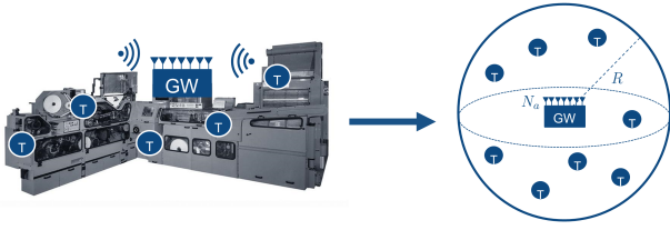
Fig. 1. The reference automation machine has tags (T) uniformly distributed inside it, that sends the collected data in uplink to the GW. Tags have only one antenna, while the GW has several antenna elements. This IIoT scenario is modeled as a 3D sphere of radius R , with the GW in its center and the tags distributed inside it.
