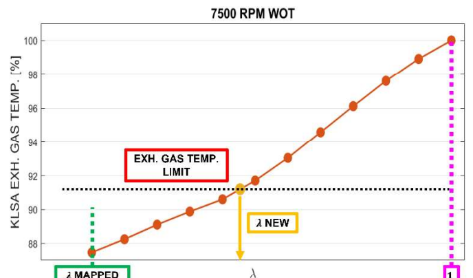
Figure 22. Trend of the exhaust gas temperature for the KLSA as a function of lambda.
