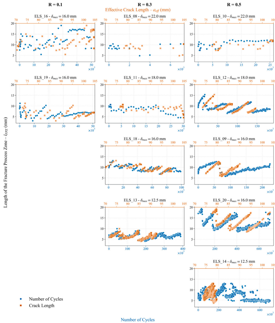
Fig. 7. Length of the fracture process zone ( l_{FPZ} ) determined by combining 2D and 3D DIC data as a function of effective crack length (orange axis) and number of cycles (blue axis) divided by R-ratio. (For interpretation of the references to colour in this figure legend, the reader is referred to the web version of this article.)
