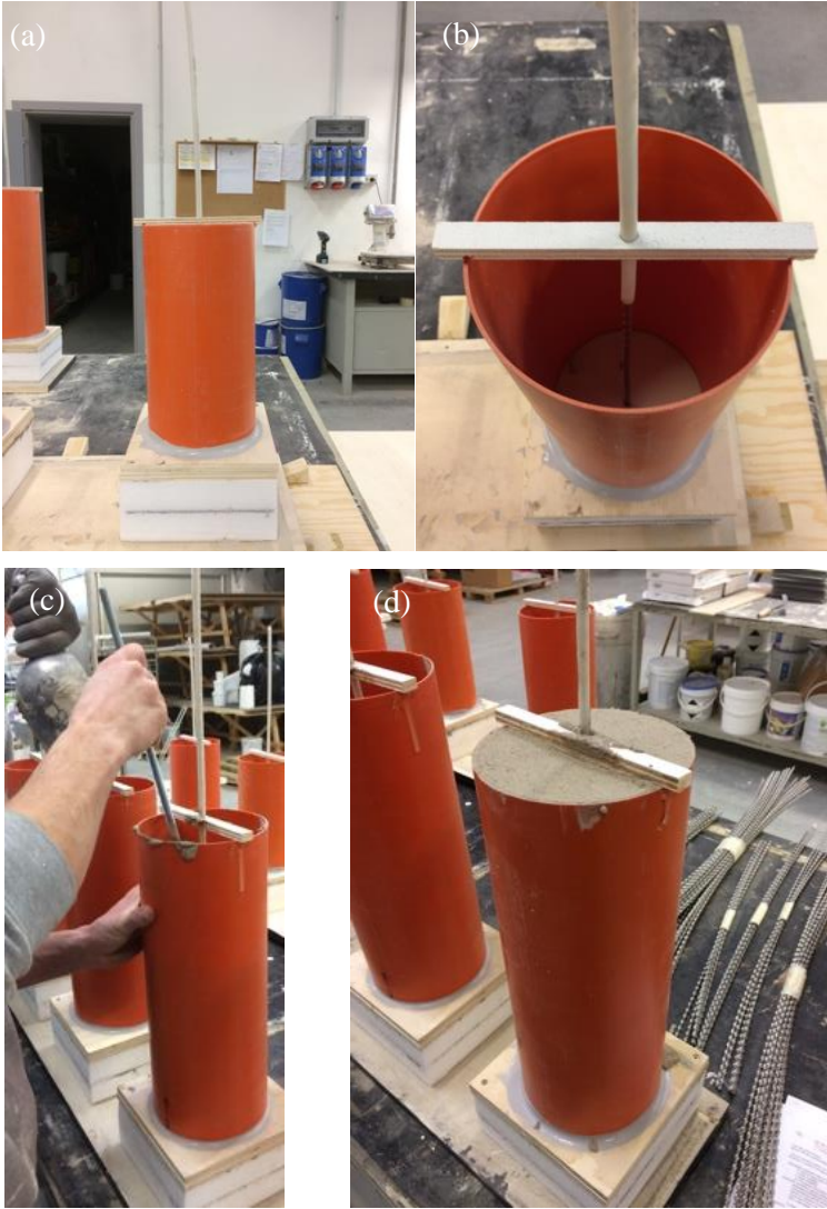
Figure 4. Construction phases of the cylindrical specimens: a) and b) the bar is positioned concentrically in the cylinder mold, a plastic tube is used to create a bond break of length equal to 50 mm from the top face of cylinder, c) mortar_s is manually rodded in order to avoid the formation of large voids, and d) the cylinders are left to cure in lab conditions.
