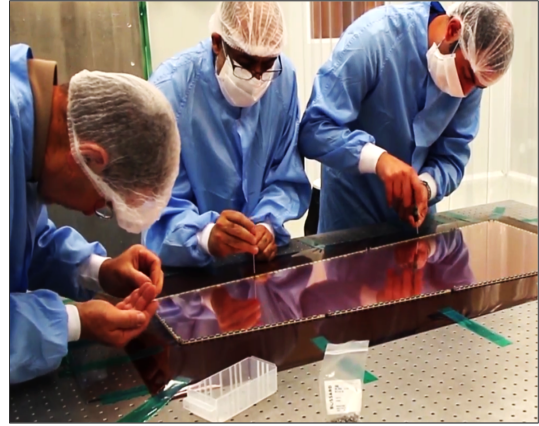
(b) Securing the GEM stack.
