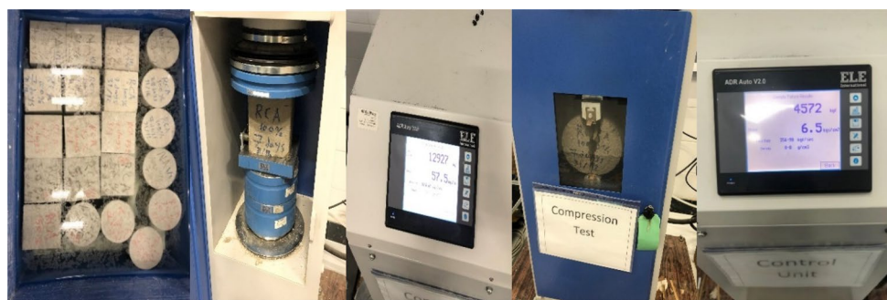
Fig. 6 Curing of samples and compressive strength and indirect tensile strength tests
