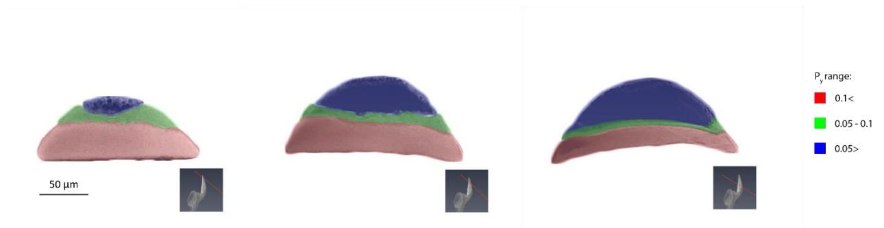
Figure S10: Topographic scan planes taken from Figure 6 and overlaid with selected average P_y ranges calculated using values for E and H , as obtained from nanoindentation. Overall wearability of the tooth decreases as a function of height leading to the conclusion that there would be a preferential self-sharpening effect as rasping occurs.
