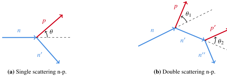
Figure 2: Neutron-proton scattering events: (a) single scattering and (b) double scattering.
