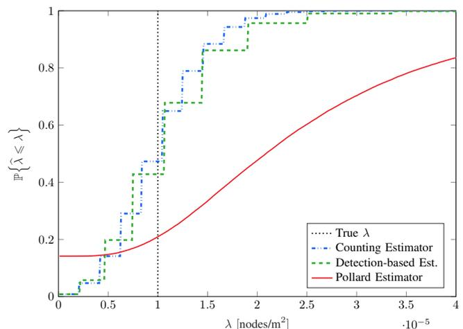
Fig. 5. Cumulative distribution functions of density estimates for  $M = 10$ ,  $\sigma_{\text{dB}} = 6$ , and  $\lambda = 10^{-5}$  [nodes/m<sup>2</sup>].
