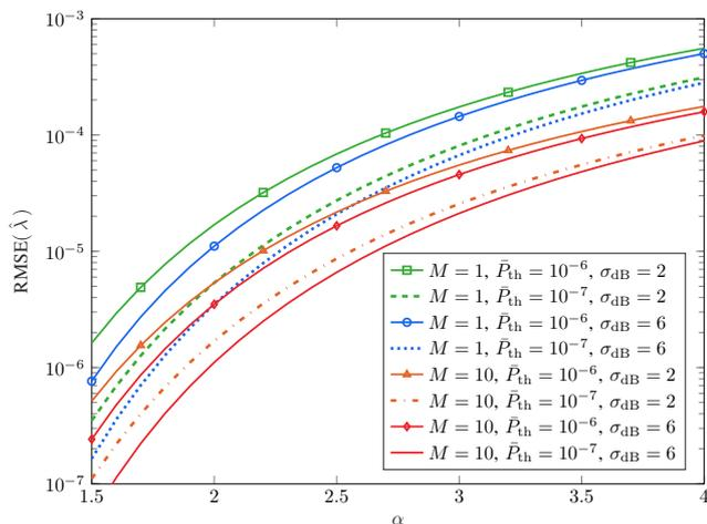
Fig. 4. Counting estimator RMSE as a function of the path-loss exponent for  $\lambda = 10^{-3}$  [nodes/m<sup>2</sup>].
