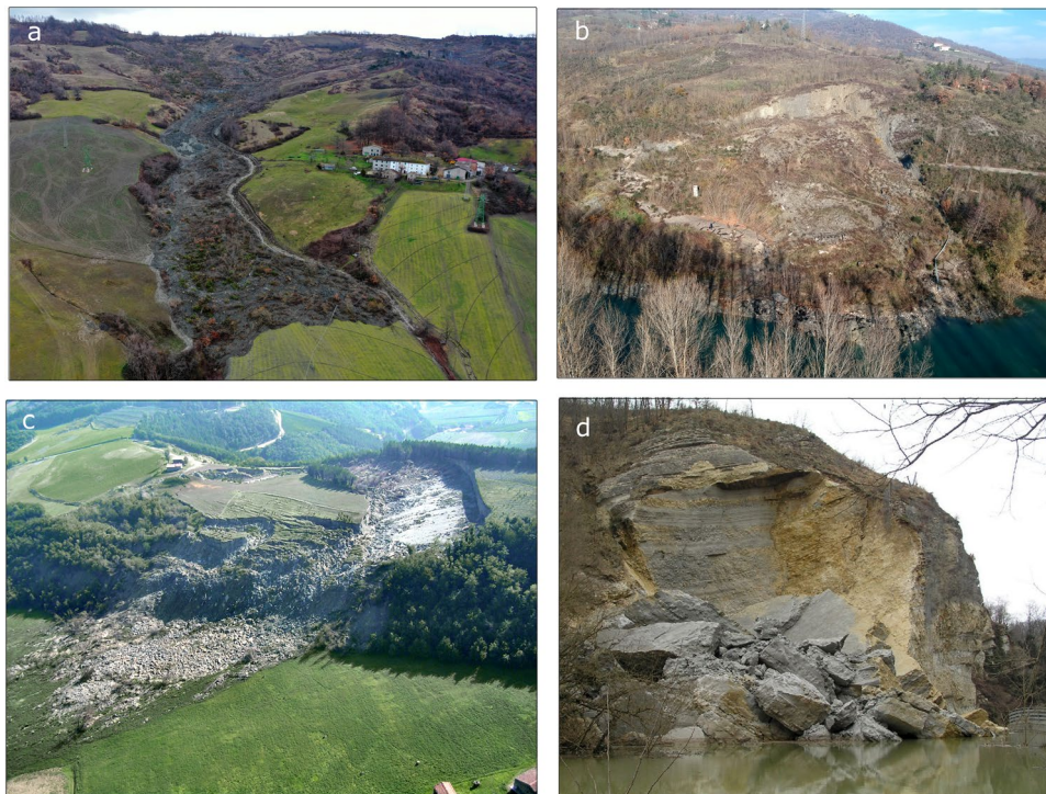
Fig. 2 Examples of landslide types in the Emilia-Romagna Region. a Earthflows and b earth slides, commonly found in the clay rocks of the Ligurian Domain. c A typical rockslide observed in the flysch rocks of the Tuscan-Romagna Domain. d Rockfall characteristic of the sandstone rocks in the Epiligurian Domain
