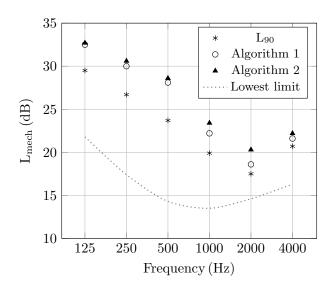
FIG. 6. Inferred values of the noise source identified as mechanical using Algorithms 1, Algorithm 2 compared with measured  $L_{90}$  in the office under study. The dotted curve shows the lowest detectable limit of the equipment used.
