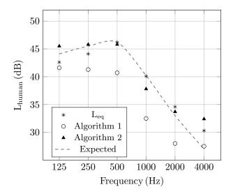
FIG. 5. Spectral matching between the calculated speech level in the room (under a diffuse sound field assumption; dashed line) and inferred values of the noise source identified as human using Algorithms 1 and 2 in the office under study. The dashed line is plotted assuming the speech running for the 20% of the monitoring time.
