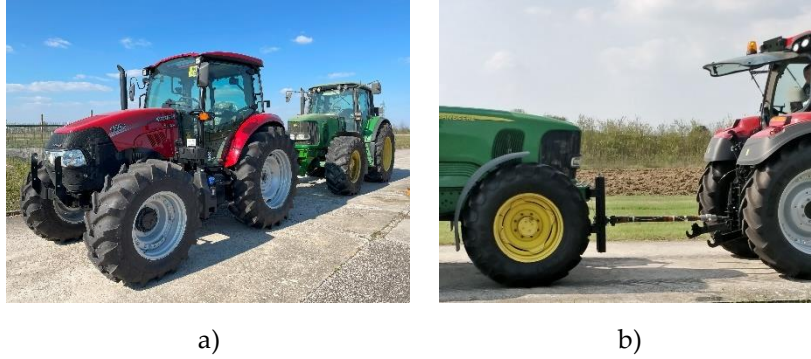
Figure 2. The traction test: a) pulling tractor with a braking tractor, b) load cell.
