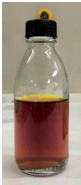
FIG. 4.1. Filtered water of sulphur (quicklime to sulphur ratio: 2:1, water). Laboratory of the Chemistry Department, Bologna. Picture by G. Montanari.
