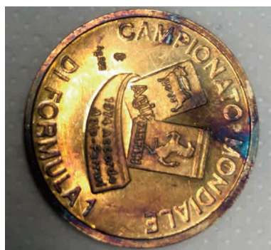
FIG. 4.4. Colouring of a silver coin dipped into the water of sulphur that has been boiled twice and filtered (quicklime to sulphur ratio: 2:1; water). Laboratory of the Chemistry Department, Bologna. Picture by G. Montanari.
