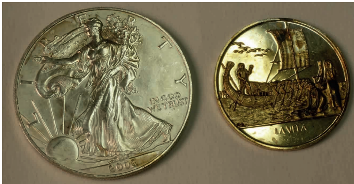
FIG. 3.1. Colouring of silver coins dipped into the water of sulphur (quicklime to sulphur ratio: 1:2; water). Laboratory of the Chemistry Department, Bologna. Picture by M. Marchini.
