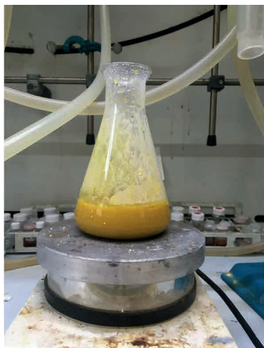
FIG. 2. Initial boiling of the water of sulphur (quicklime to sulphur ratio: 1:1; vinegar). Laboratory of the Chemistry Department, Bologna. Picture by M. Marchini.
