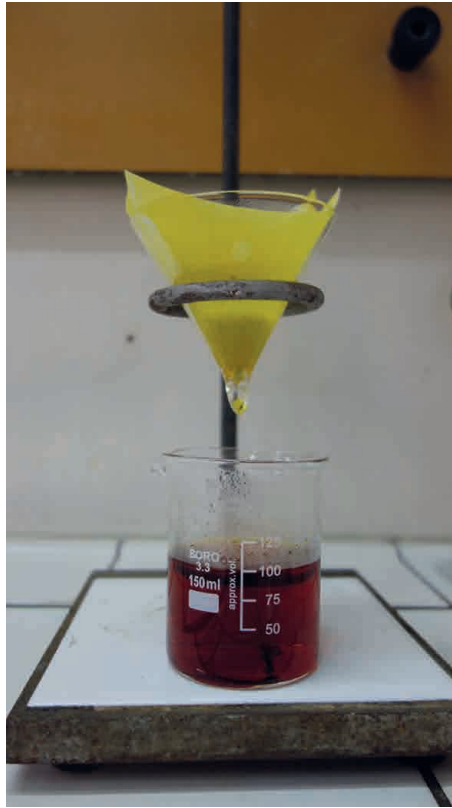
FIG. 3. Filtered water of sulphur (quicklime to sulphur ratio: 1:2; water). Laboratory of the Chemistry Department, Bologna. Picture by M. Marchini.
