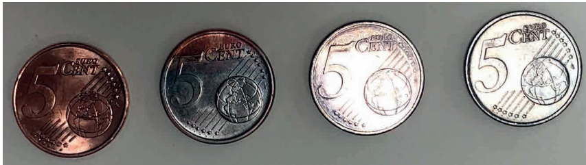
FIG. 8.1. Various shades of silver on copper coins dipped into Pseudo-Democritus' wash prepared with filtrate of quicklime (L). Laboratory of the Chemistry Department, Bologna. Author's picture.
