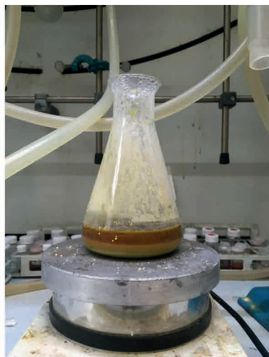
FIG. 2.1. Water of sulphur gently boiled for 30 minutes (quicklime to sulphur ratio: 1:1; vinegar). Laboratory of the Chemistry Department, Bologna. Picture by M. Marchini.
