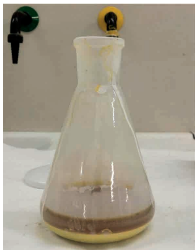
FIG. 4.2. Filtrate of the water of sulphur boiled again in water (quicklime to sulphur ratio: 2:1, water). Laboratory of the Chemistry Department, Bologna. Picture by G. Montanari.
