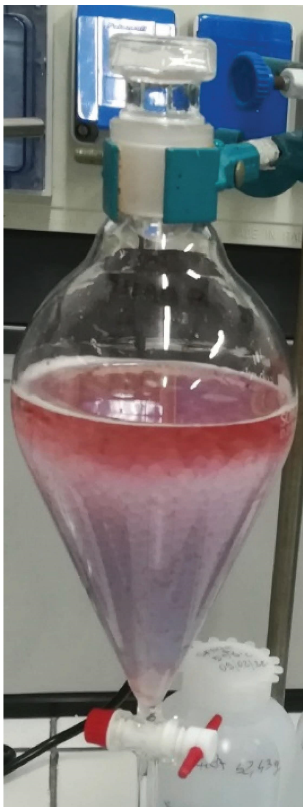
FIGURE 4 | Rosé wine in the separating funnel in contact with the TiO 2 paste-coated glass spheres.
