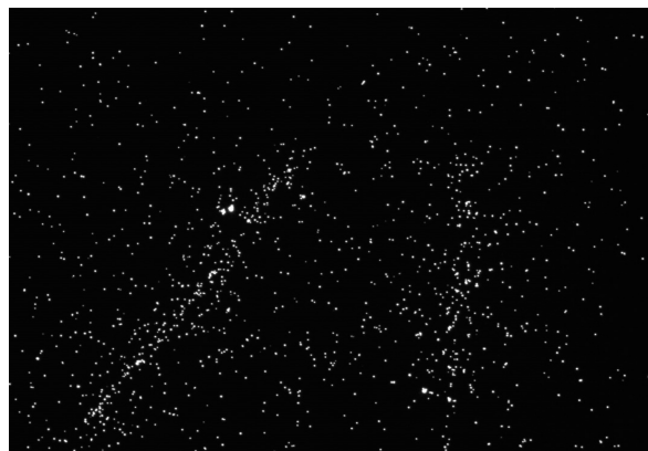
Figure 4. Example of a MIP event: the left panel shows a track produced by a cosmic muon in the CsI(Tl) scintillator, while the right panel displays the corresponding mirrored image.
