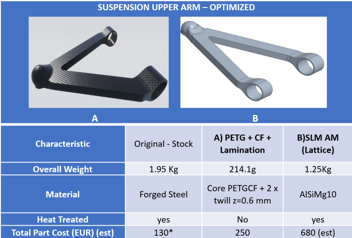
Figure 11. Lightened part in AM versions, carbon fiber PETG (A) and SLM (B) and key technical achievements. * Production tooling cost not accounted.
