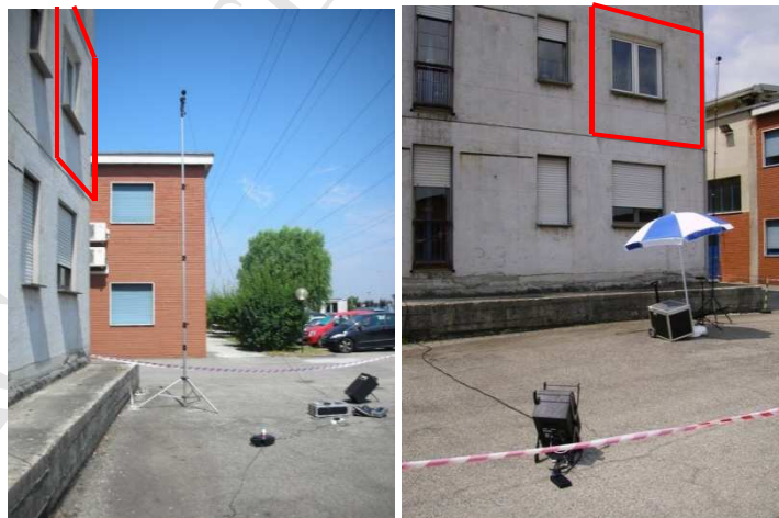
Figure 1. Different loudspeaker positions: on left side in front of the facade, on right side in a lateral position. Contoured in red the test facade.
