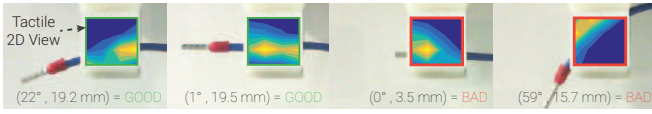
(a) The binary classifier distinguishes between Good (1) and Bad (0) grasps using tactile sensor measurements.
