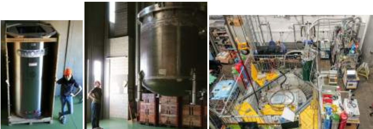
Figure 17. (Left) The cryostat for testing Module 0. (Center) The cryostat for the ArgonCube 2 \times 2 Demonstrator. (Right) The 2 \times 2 cryostat and cryogenics system at the Univ. of Bern.
