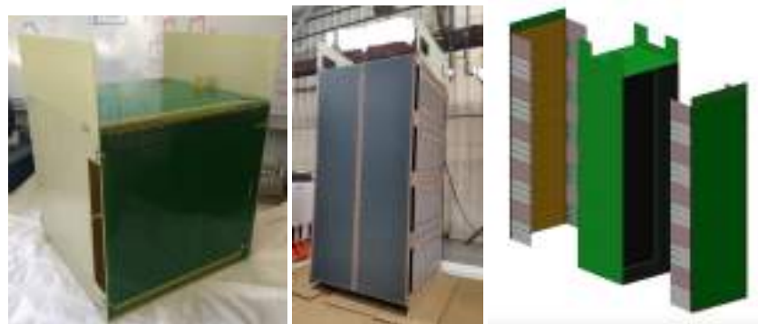
Figure 14. (Left) The SingleCube LArTPC designed to test a single integrated large-format charge and light readout element. (Center) The mechanical assembly of the first module (Module 0) of the ArgonCube 2 \times 2 Demonstrator, including the cathode, field cage, and anode support panels. The module is a sub-scale prototype of the ND LArTPC module, at 60% drift length and 40% module height. (Right) The engineering model of the full-scale ND LArTPC module (1 m by 1 m footprint and 3.5 m height), shown with the anode panels detached from the field cage. The pixelated anode tiles (gold rectangles) provide true 3D imaging, while the dielectric light traps (pink and white rectangles) provide high-efficiency scintillation light detection.
