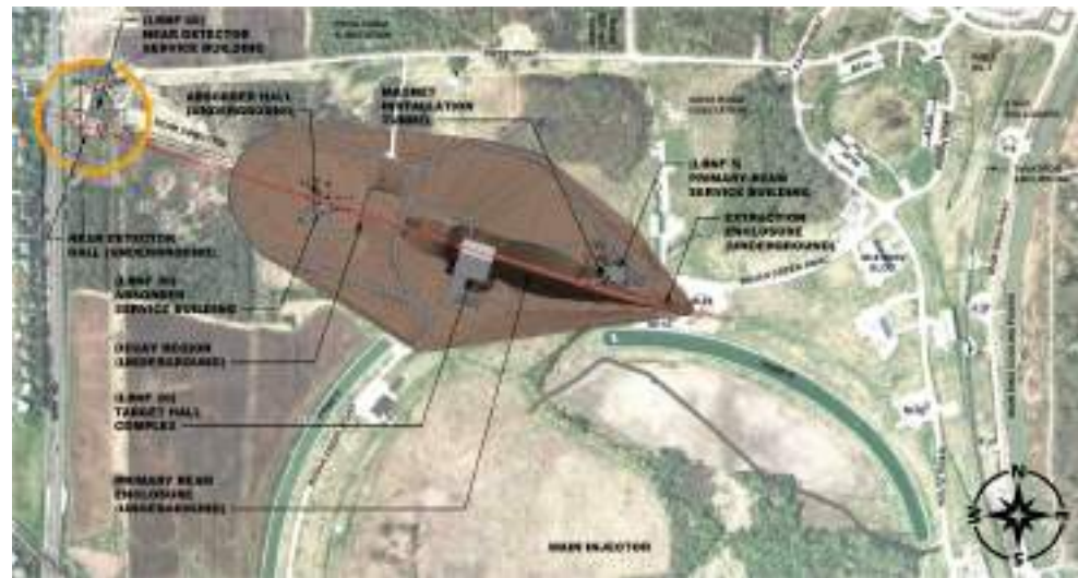
Figure 164. Birds-eye view of the future LBNF/DUNE construction site. The Near Detector cavern will be located at the west-most boundary of Fermi National Lab.
