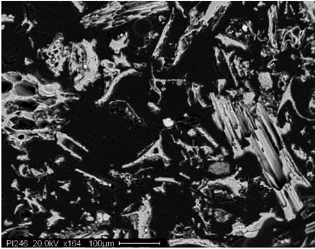
Fig. 4 Scanning electron microscope image of Oscurusciuto tephra, showing both aphyric glass shards and vesicular micro-pumice fragments
