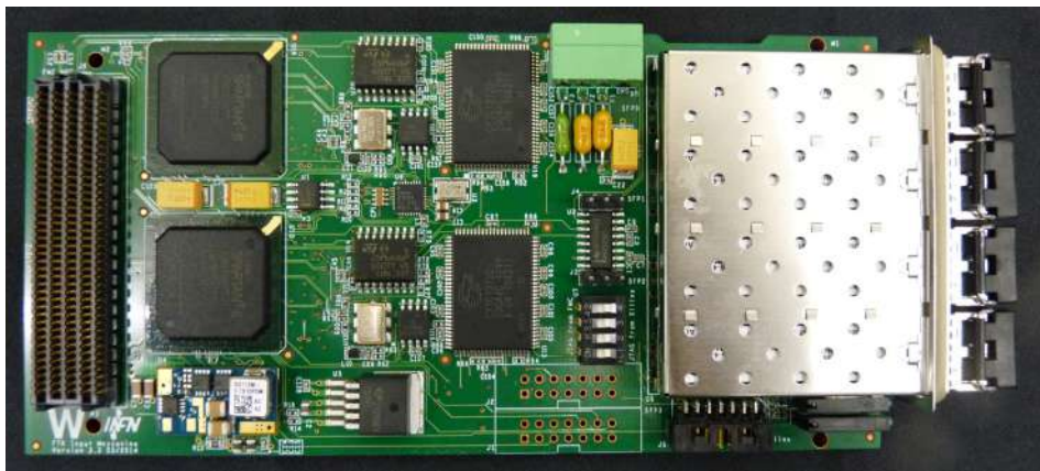
Figure 5. Photo of the Spartan-6 Input Mezzanine card, component side.
