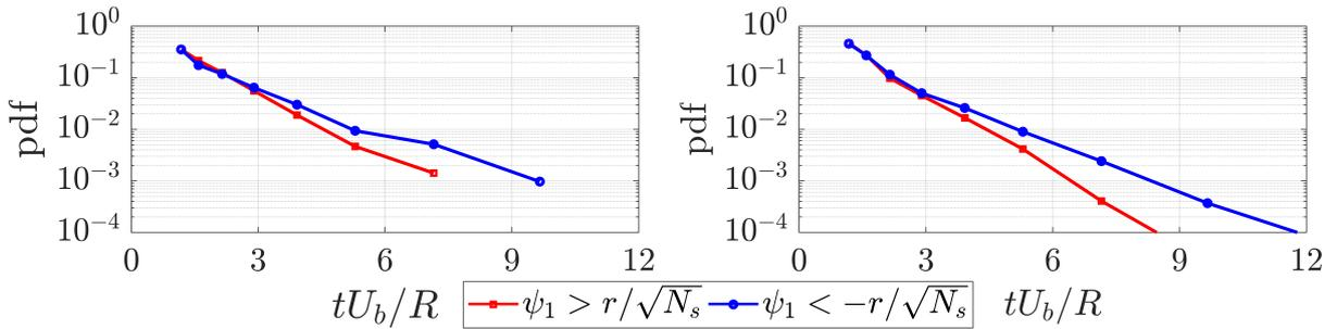
Figure 8: Statistical distribution of large scale motions. Left:  $Re_\tau = 9500$ . Right:  $Re_\tau = 20000$ . Events with large positive/negative values of the first time coefficient indicate high/low momentum structures.
