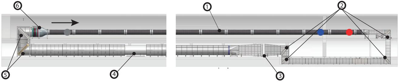
Figure 1: Overview of the Long Pipe (LP) facility: 1) The carbon-fiber pipe 2) Rectangular expanding corners 3) Heat Exchanger 4) Fan assembly 5) Round corners 6) Settling chamber and Convergent assembly. The arrow shows the flow direction. The red, blue and gray markers indicate the location of the measurement station, of the Pitot tube and the PIV seeding particles inlet, respectively.
