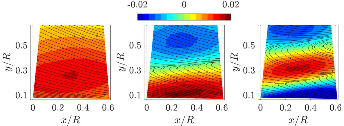
Figure 4: POD spatial modes of the velocity fields (left: 1st; center: 2nd; right 3rd), for the test case with  $Re_\tau = 9500$ . The contour represents the streamwise velocity component of the POD modes with superposed streamlines indicating the streamwise-radial velocity components.
