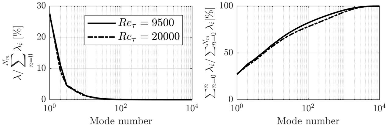
Figure 3: Distribution of POD eigenvalues (left) and their cumulative eigenspectrum (right).
