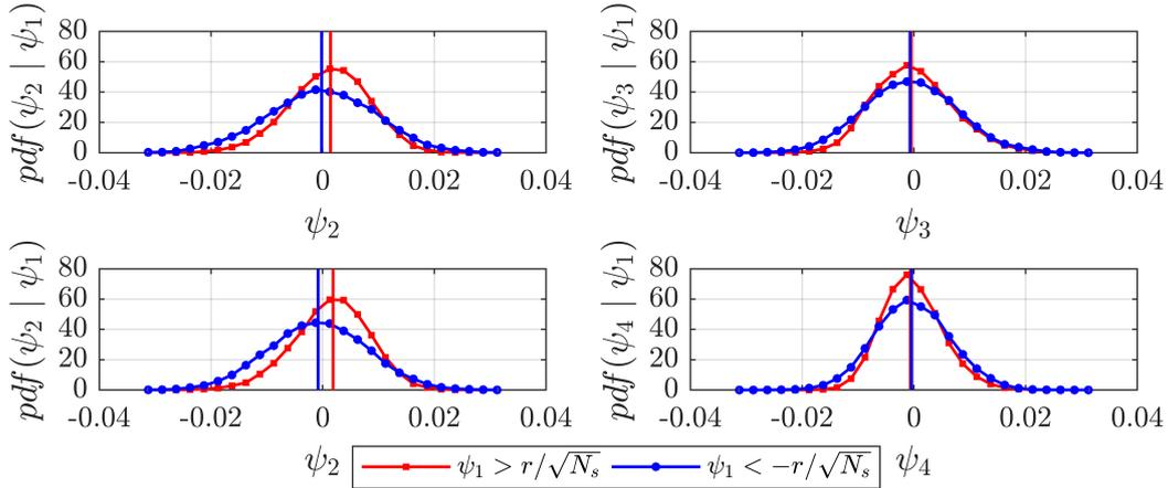
Figure 9: Conditional pdf (based on the sign of the LSM detection criterion) of the time coefficients of the  $2^{nd}/3^{rd}$  mode (top:  $Re_\tau = 9500$ ) and  $2^{nd}/4^{th}$  mode (bottom:  $Re_\tau = 20000$ ). For the case of  $Re_\tau = 20000$  the  $4^{th}$  mode has a similar spatial organization of the  $3^{rd}$  mode for  $Re_\tau = 9500$ , and for this reason it is selected herein for comparison.
