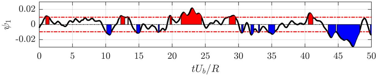
Figure 7: Identification of persistent high/low momentum structures using the first time coefficient. The sequence is from the test case with  $Re_\tau = 9500$ . Red/blue shadowed areas indicate high/low momentum structures, respectively. Dashed lines indicate the cutoff level to consider the event as high/low momentum.
