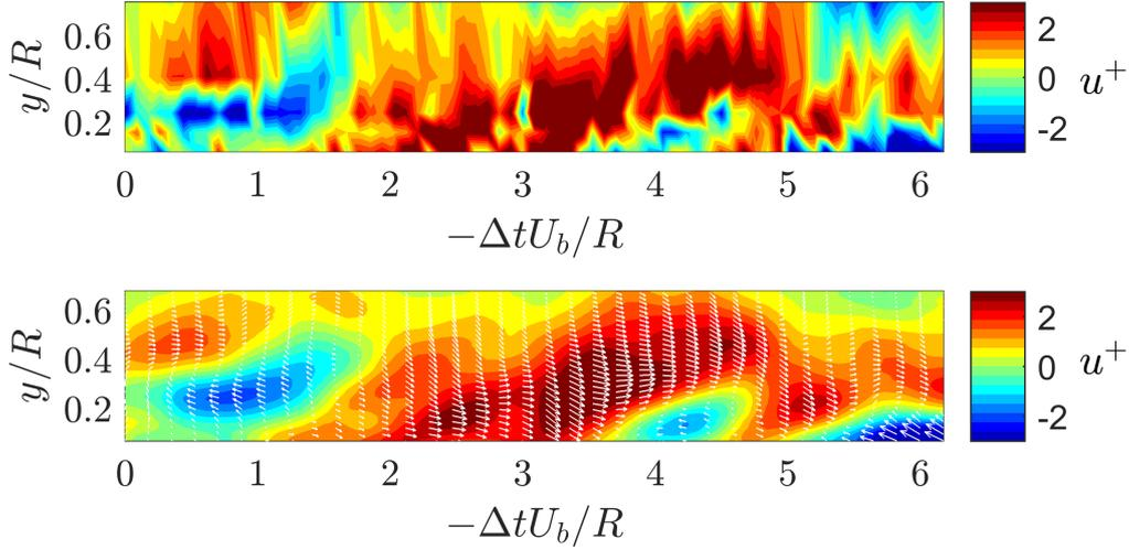
Figure 6: Contour of the evolution of the streamwise velocity component obtained using Taylor's hypothesis for the test case with  $Re_\tau = 9500$ . Top: hot-wire data. Bottom: dynamically-estimated fields. The velocity contours are shown in inner units, i.e.  $u^+ = u/u_\tau$ .
