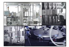
Fig. 1 - Examples of rotary tables used for capping machines and tablet press machines. Photo gently provided by IMA Group.
