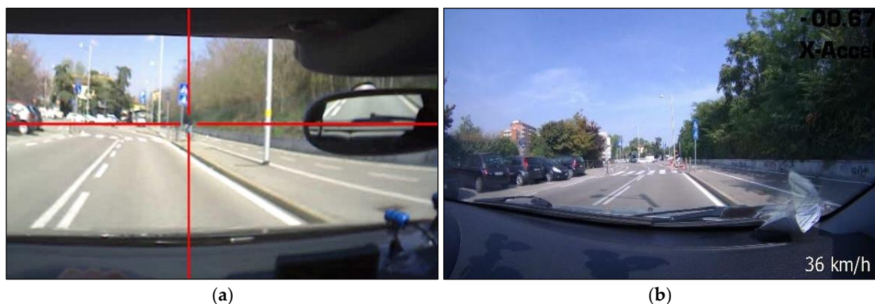
Figure 4. Synchronization of the eye-tracking mobile video output with the Video VBOX video output. (a) Video of the ME with the point of fixation (red cross), (b) Video of Video VBOX.
