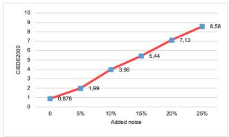
Fig. 10.  $\Delta E_{00}$  variation increasing the amount of the noise.
