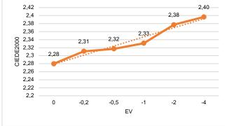
Fig. 8. The effects of exposure on development results.
