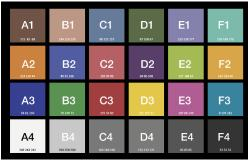
Fig 1. The target Calibrite ColorChecker Classic.
