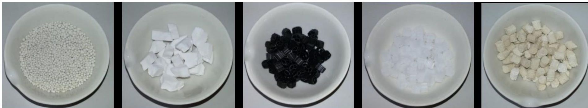
Figure. S1. Pictures of the five tested carriers. From left to right: Poraver ® , Glaxstone ® , Bio-Flo 9 Sinker ® , Kaldnes K1 ® , Biomax ® .
